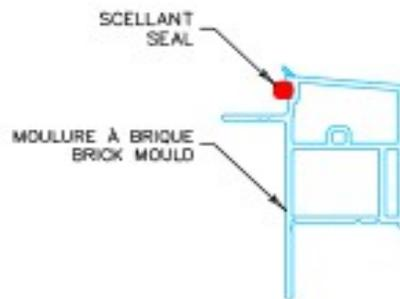
The application of the sealant under the M.A.B is the most important step in order to prevent any water infiltration.
